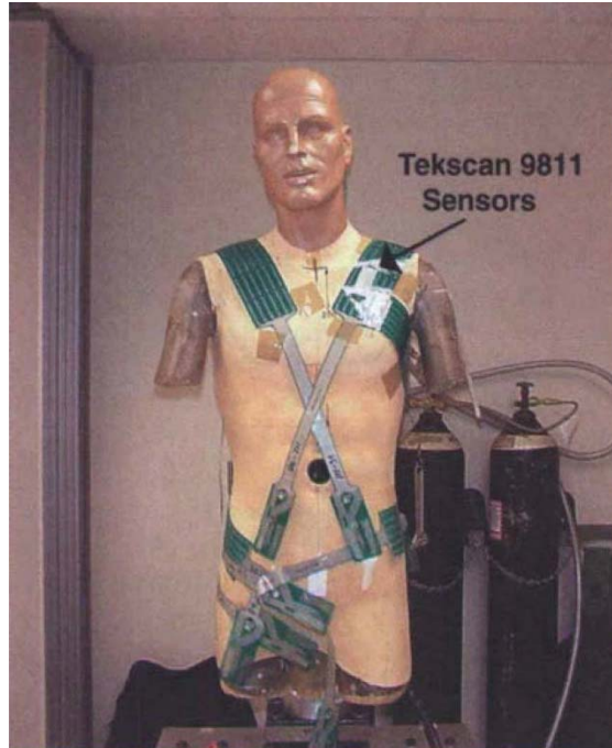
Figure 2.2 F-Scan™ pressure sensors placed onto the Dynamic Load Carriage Simulator. [52]
