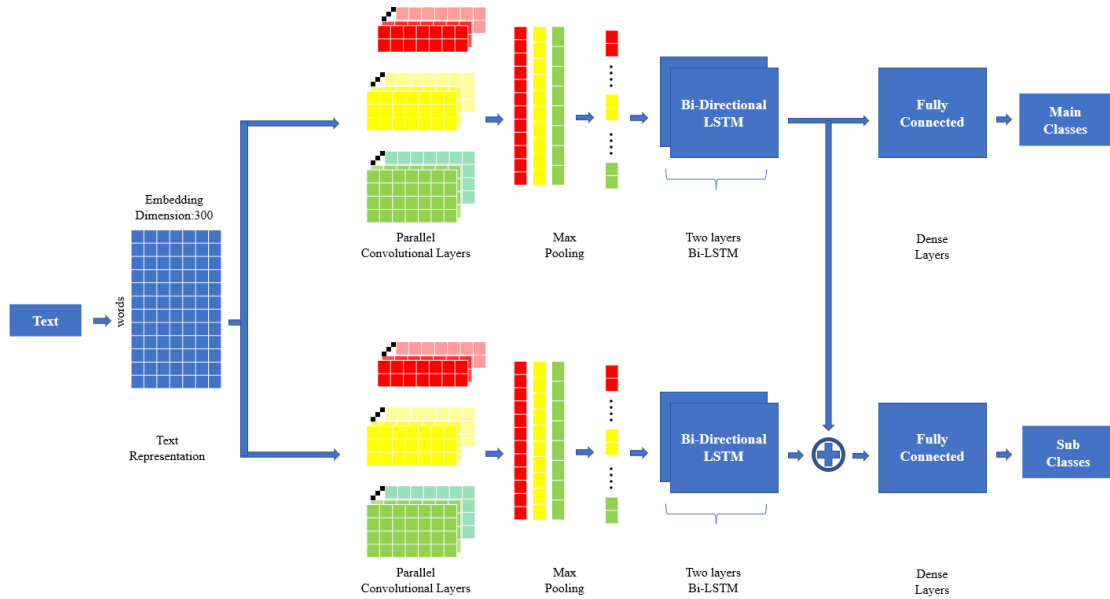
Figure 3.5: Hierarchical CNN-BiLSTM model structure
