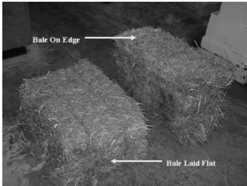
Figure 1.6: Bales Laid Flat and on Edge
