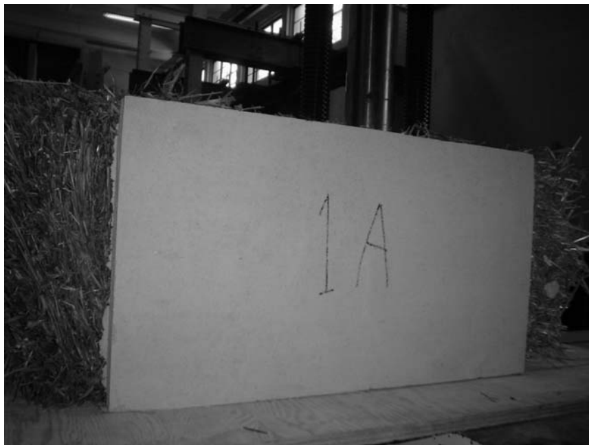
Figure 4.5: Completed Plastered Bale
