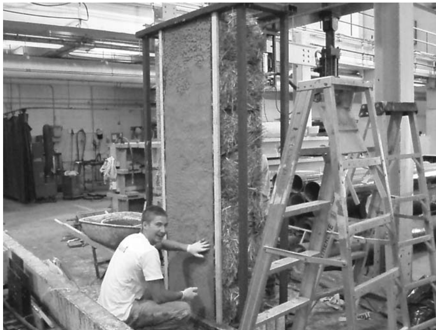
Figure 5.2: Fabrication of 2.31 m Wall Using Testing and Fabrication Jig
