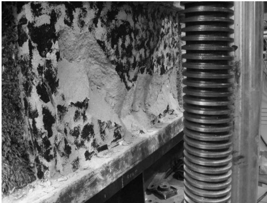
Figure 6.11b: Failure of Specimen E12
