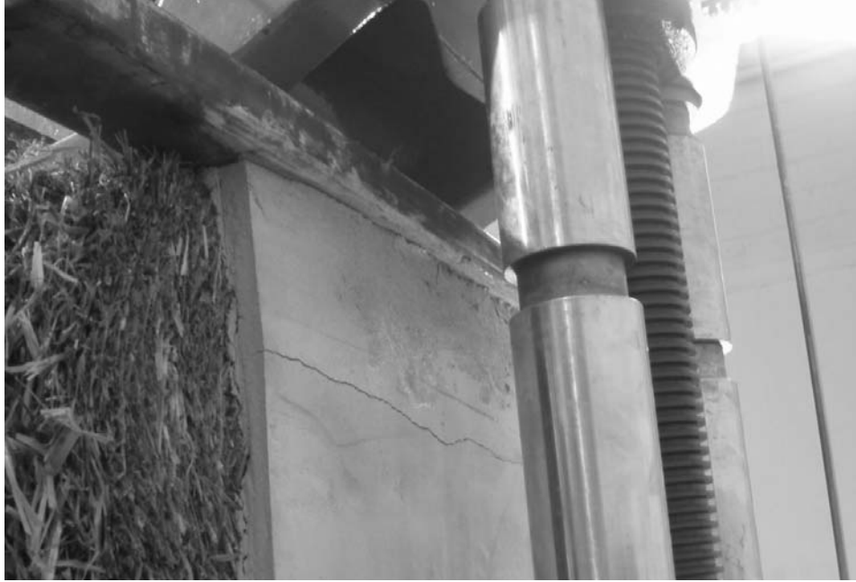
Figure 6.23: Tensile Failure of Second Plaster Skin
