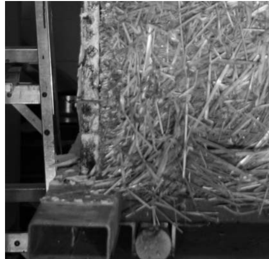
Figure 6.15b: Failure of Specimen E33
