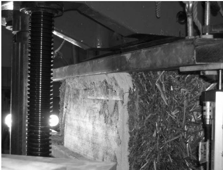
Figure 6.16b: Failure of Specimen C11
