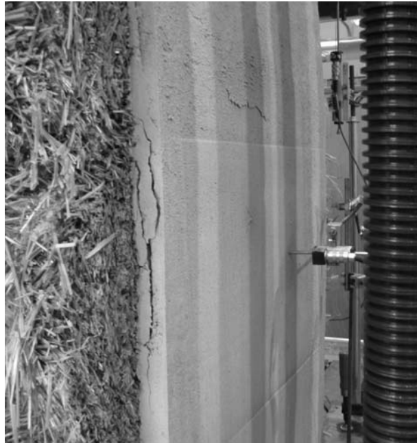
Figure 5.27: Progressive Failure of Plastered Straw Bale Wall Assemblies
