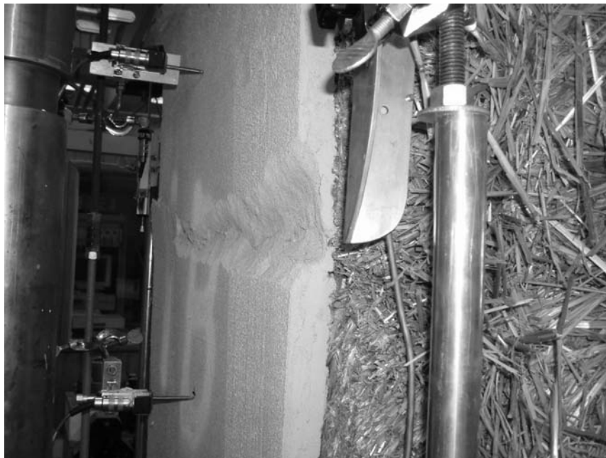
Figure 5.26: Typical Compression Failure of Plastered Straw Bale Wall Assemblies
