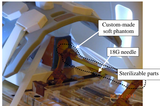
Figure 4.6: Needle placement in a soft phantom for measuring of the robotic system total error and the artifact shift. CIRS 053 prostate phantom was customized to eliminate needle deflection.
