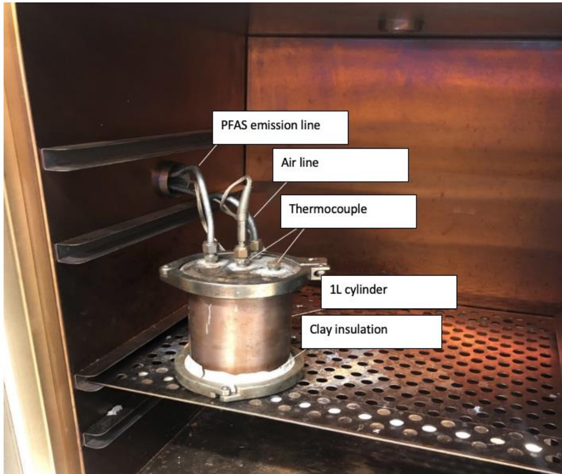
Figure A.1: Cylinder unit holding PFAS-contaminated sand, with PFAS emission line, air line, and thermocouples connected to the top plate. Clay insulation was used to minimize the leakage.
