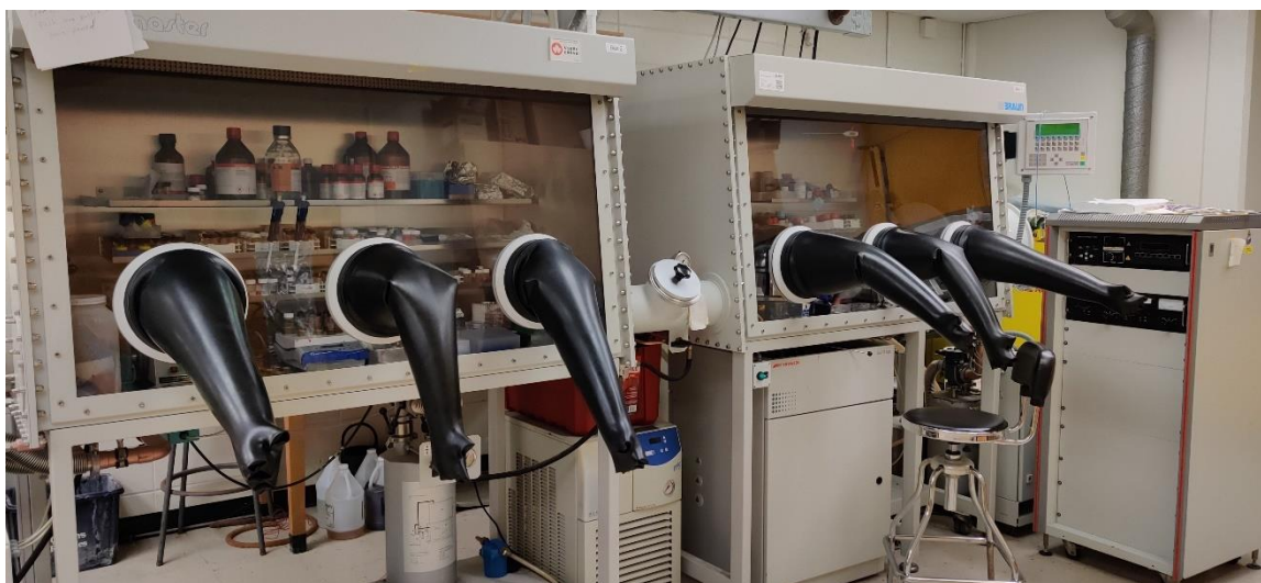
Figure 3.1 MBraun inert atmosphere glovebox/evaporator system.
