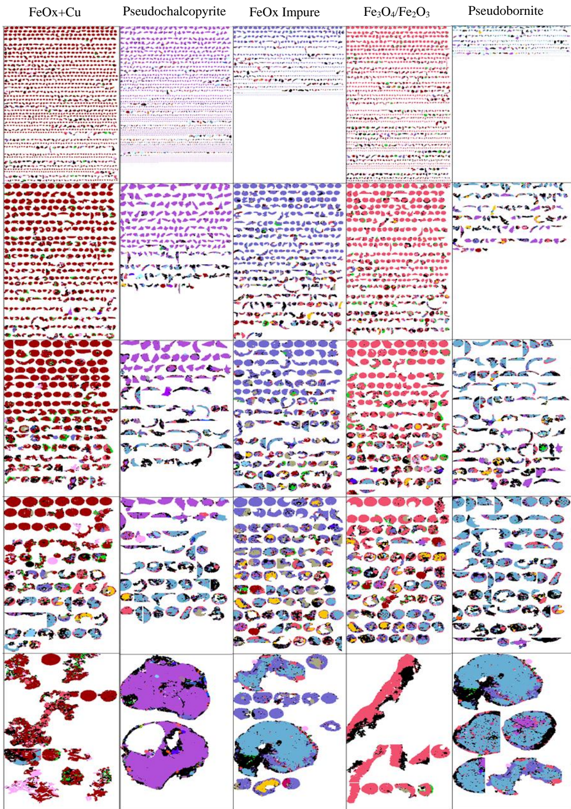
Figure 11: QEMSCAN® mineralogical map for Concentrate A with O 2 /S = 1.9
