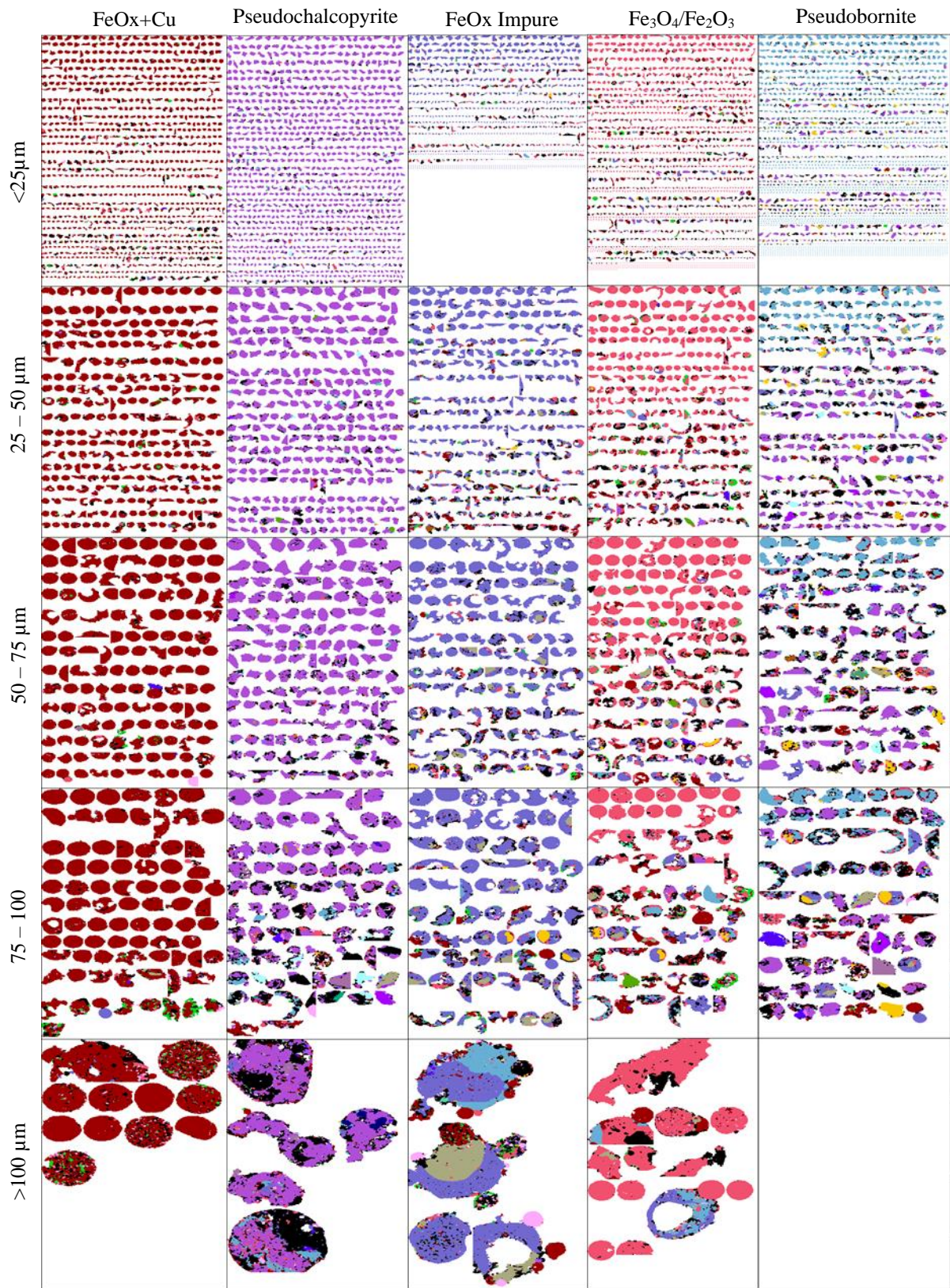
Figure 13: SEM-EDS QEMSCAN® mineralogical map for Concentrate B with O 2 /S = 1.9
