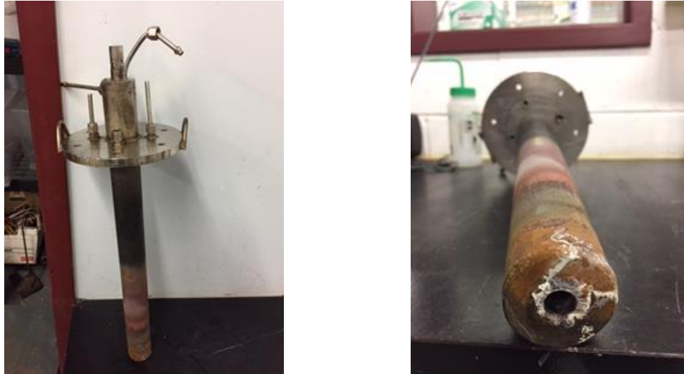
Figure 5: Solids feed lance – front and bottom views
