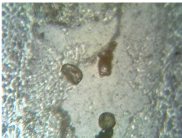
Fig.5.9. The gap on the surface of the partly degraded acrylic layer on the 14 th day of incubation. The dark border along the gap is the colonies of bacteria. Germinated fungal spores are located in the gap. The slide was contaminated in the storage facility. Magnification 40X.
