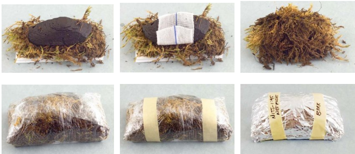
Fig.2.7. A fragile bark net float is supported by a piece of coroplast, cushioned by a layer of Sphagnum moss, wrapped in plastic film to prevent drying, wrapped in aluminum foil, and finally securely taped with the identification records (photos from Scott and Grant 2007).
