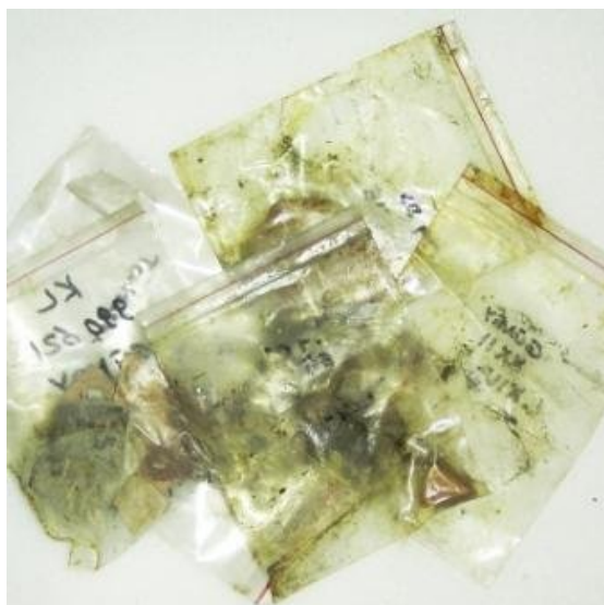
Fig.5.2. Polyethylene bags used to store small bronze objects after microbial attack. The black spots are due to colonies of Aspergillus niger . Artifacts have been removed.
