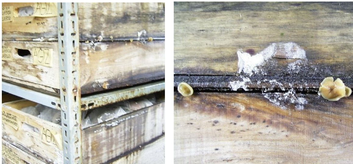
Fig.5.1. Mould- infested wooden boxes holding ceramic artifacts in the Kaman- Kalehöyük storage site-on the left. The variety of fungal spp. on the surface of a box -on the right (magnified). In this image two fruit bodies of white rot fungi can be seen. The black spots are due to colonies of Aspergillus niger .
