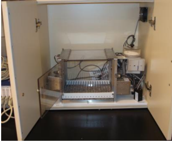
Figure 2. Operant conditioning box within a sound-attenuating cabinet.
