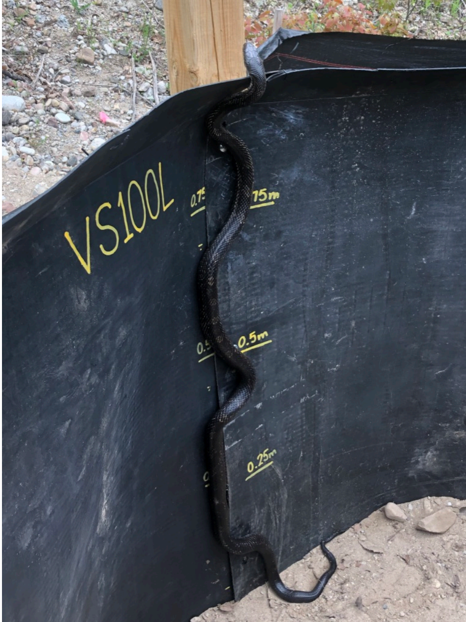
Figure 8. Gray ratsnake ( Pantherophis spiloides ) using the vertical seam of the fence during its escape from 100 cm vinyl sheeting with a lip.
