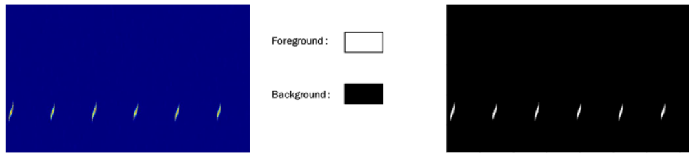
Figure 3.4: Foreground and background separation of the STFT plot of a given signal.
