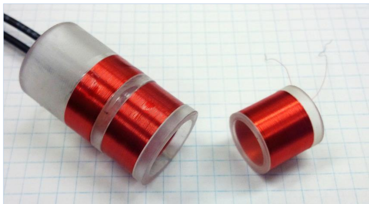
Figure 16: Tandem driver-pickup tube probe (left) and encircling driver-pickup rod probe (right).
