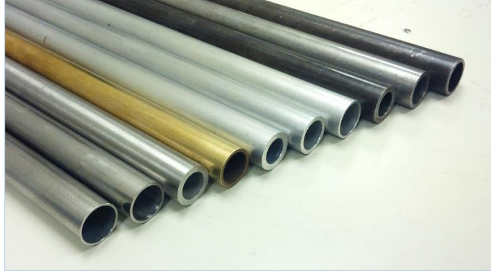
Figure 17: Assorted aluminum, stainless steel, brass and carbon steel tubes with \frac{3}{4} " outer diameter.
