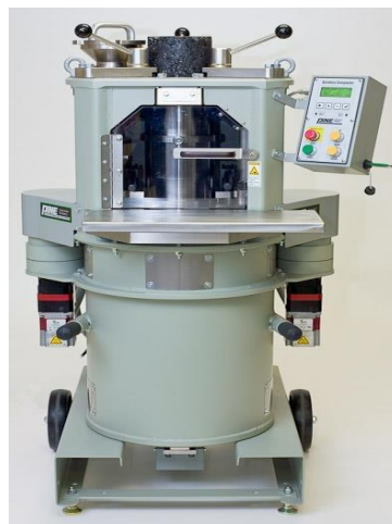
Figure 2.19: Pine Instruments Superpave Gyrotory compactor (SGC) [60].
