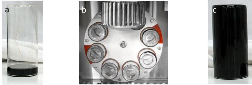
Figure 3.1: RTFO aging. A) Loading the glass tube, b) Rolling in RTFO and c) coated tube after aging [75].
