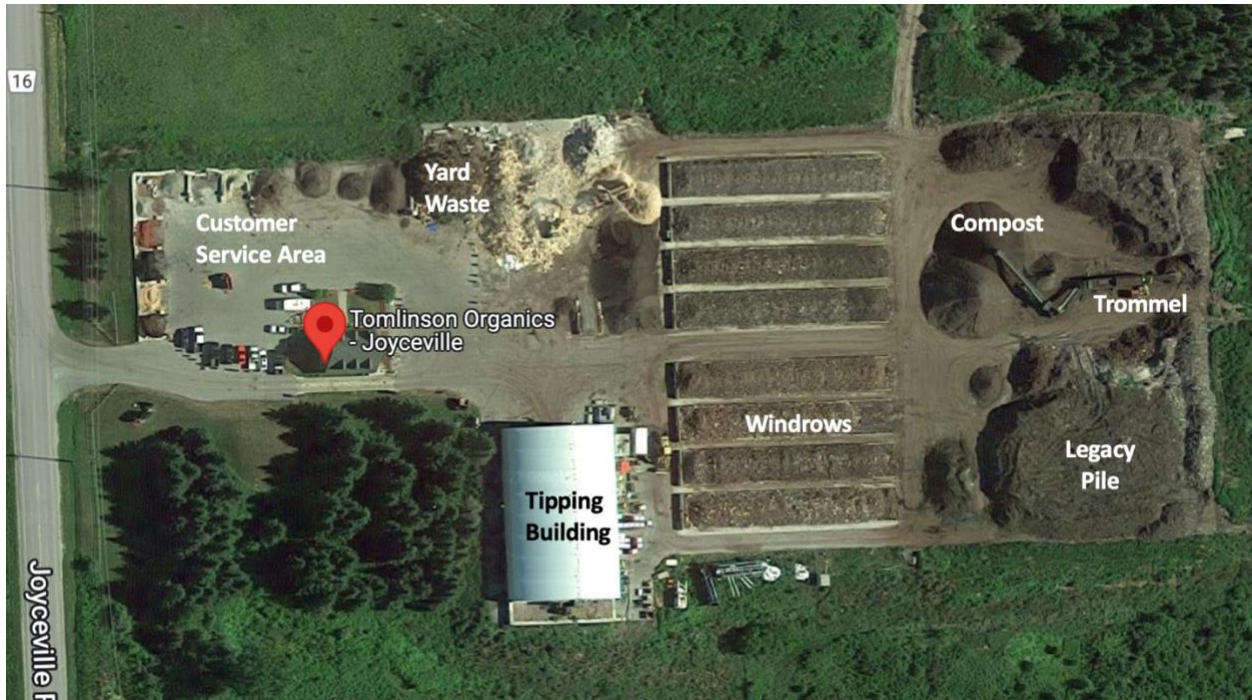
Figure 6: Tomlinson Organics, Joyceville, Ontario. Source: Google maps, satellite view, unknown year, labels added by author. There are currently more legacy piles than pictured.
