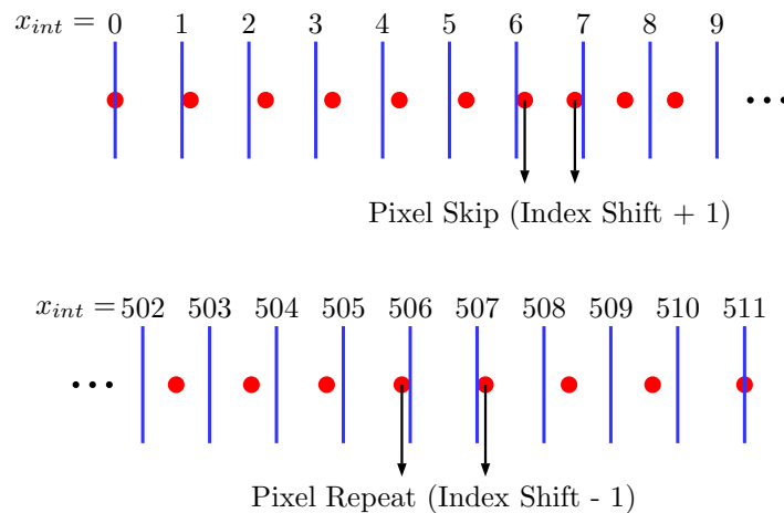
Figure 3.6: Visualization showing the unevenly sampled raw signal x -values as red dots and the evenly spaced resampled x -values as blue lines. The case where two raw spectrum values fall between consecutive interpolated values is shown on the top, and the case where two interpolated values fall between consecutive raw spectrum values is shown on the bottom.
