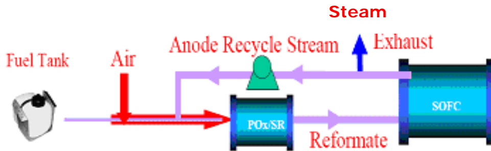
Figure 1.5: Schematic of fuel cell-powered APU system
